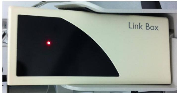
**\*The red light should be blinking when the software is not loaded. When the software is loaded the link box should show a solid red light.**
